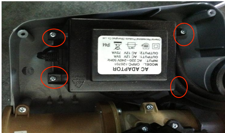
11. Unscrew the screws that fix the transformer onto the control box.
