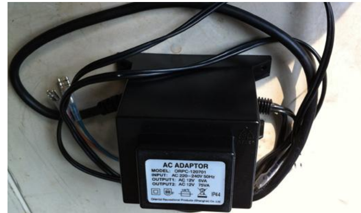
12. Take out the original transformer from control box and install the new transformer in reverse order.
